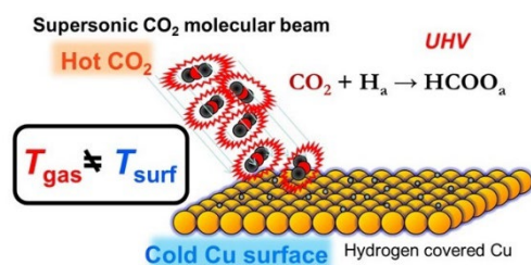
Fig.1 Reaction takes place by supplying vibrational energy only to CO 2 without heating a Cu catalyst. Nature Chemistry ( ref.2)
