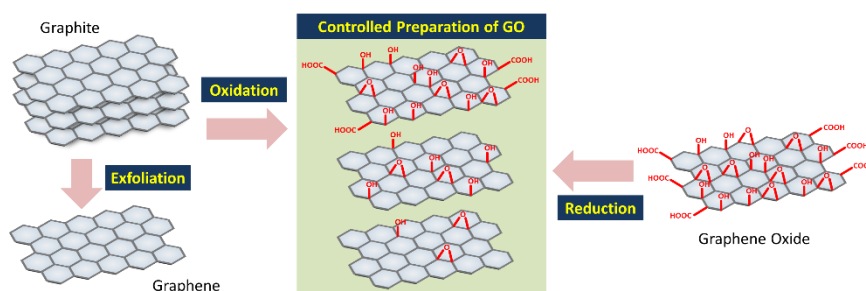
Fig. 1. Tuning the structure and oxygen content of carbon materials.
